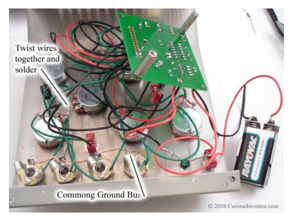
(this images is from an older version, the resistor attached to R6 is now on the PCB)
