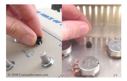
Install the LED holers from the outside, then press the LEDs into them from the inside until they snap in place.
