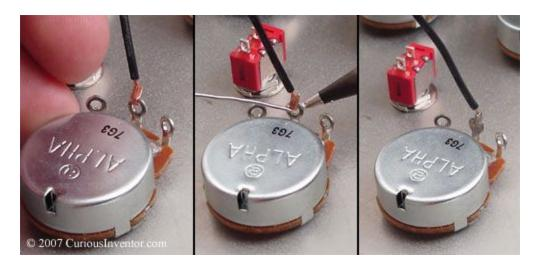
First loop the wire through and bend it to hold it in place, then heat the joint from one side and apply soder to the other. Again, it will help to put a bit of solder between the iron tip and connection to act as a heat bridge.
