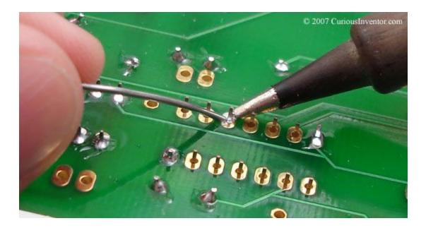
Tin the tip, or in other words, add a bit of solder to the tip, first. This small amount of solder forms a "heat bridge" to help conduct heat from the tip to the pad and component lead. When you first contact the parts with the iron tip, it's helpful to first place some solder in
