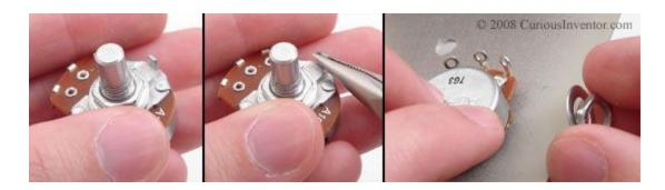
First break off the anti-rotation tab with pliers, then install like the following picture shows:
