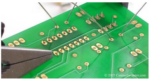
To keep components in place while you solder them, clinch (bend / splay) the leads outwards. On the IC, do this for two opposite corners. This is actually what automated machines do to keep chips in place while the boards are run over fountains of liquid solder (wave soldering).
