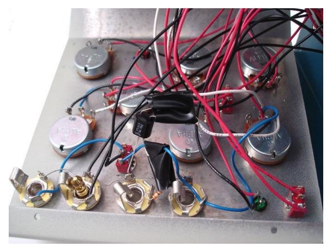
Install the vactrol and 390ohm resistor directly inside the case. Use electrical tape or heat shrink tubing to protect the wires. Make sure the positive side of the vactrol is attached to the positive Jack terminal. See the <u>connection diagram</u> for more clarification. Finally solder wires to the battery holder, attach the standoffs to the pcb and screw together the case.
