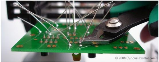
Cut off the leads as you go with flush cutters. Watch out for flying leads; safety glass are actually not over-precatious for this, although we generally just hold the lead with fingers to keep it from flying off.
